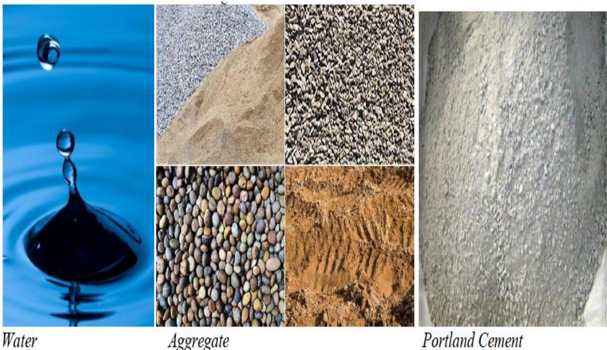
Figure 1: Synoptic View of Concrete
